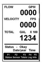
The screen at the right is the main screen for the Accuron 7700. It will display flow, velocity and totals. It will also give a status of the velocity signal crossing the pipe. An "Okay" signifies proper reception of the crossing signal. A "No signal" signifies that there are interruptions of the crossing signal and that the meter will not register flow.
