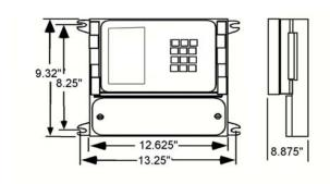
mounting feet have slots for ½" bolts (4 places). The electronics should be mounted with the display at eye level or lower. There are three ½" holes in the bottom of the enclosure for conduit fittings. These holes have rubber plugs installed at the factory. If you do not use all three holes for conduit, leave the rubber plugs in the holes to protect the enclosure ratings.
