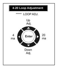
To adjust the 4-20 output, use the circular keypad. You must have a milliamp meter inline with the current output to adjust.
